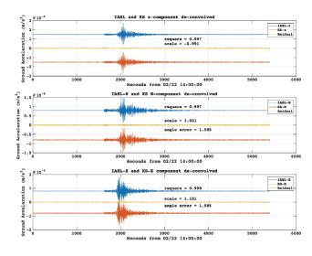
Figure 3. An example of a seismogram showing comparison between the optical seismometer, processed to convert mass position to ground acceleration, and the records from a co-located KS54000.
