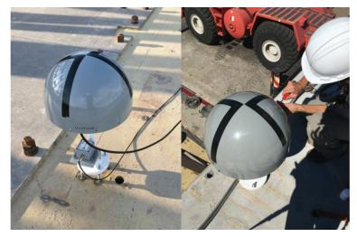
Figure 6. Installation of seismogeodetic instrumentation on a structure at the NHERI@UCSD Large High Performance Outdoor Shake Table. (Left) GPS antenna and SIO MEMS accelerometer on the shake table platen. (Right) On roof of the structure. The black tape on the antenna covers serves as targets for geoferencing UAV images of the structure, We use these earthquake simulations to test real-time data collection and earthquake detection algorithms.
