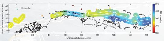
Figure 11. Map of permafrost thickness, offshore Prudhoe Bay, Alaska, measured using a novel surface-towed marine EM system developed by the marine EM lab.
