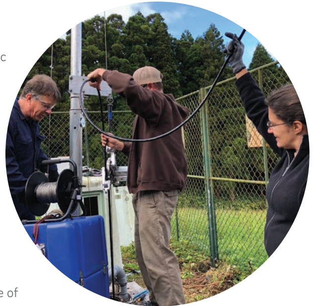
Figure 12. IDA's Chris Sites and Clint Coon prepare to lower the new STS6A seismometer into the 100m deep borehole at station II.CMLA (Chã de Macela, Azores). Station operator Maria Escuer of our host organization, the OAC, assists. Photo courtesy C. Sites.
