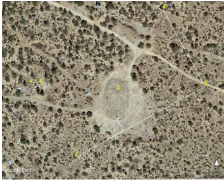
Figure 3. Map of PFO showing the locations of proposed new holes (SDF, SDG, and SDH) with yellow pins, trenches connecting these holes to existing power/communications infrastructure as white lines, and the location of two pre-existing holes (SDC, SDT) were modified.
