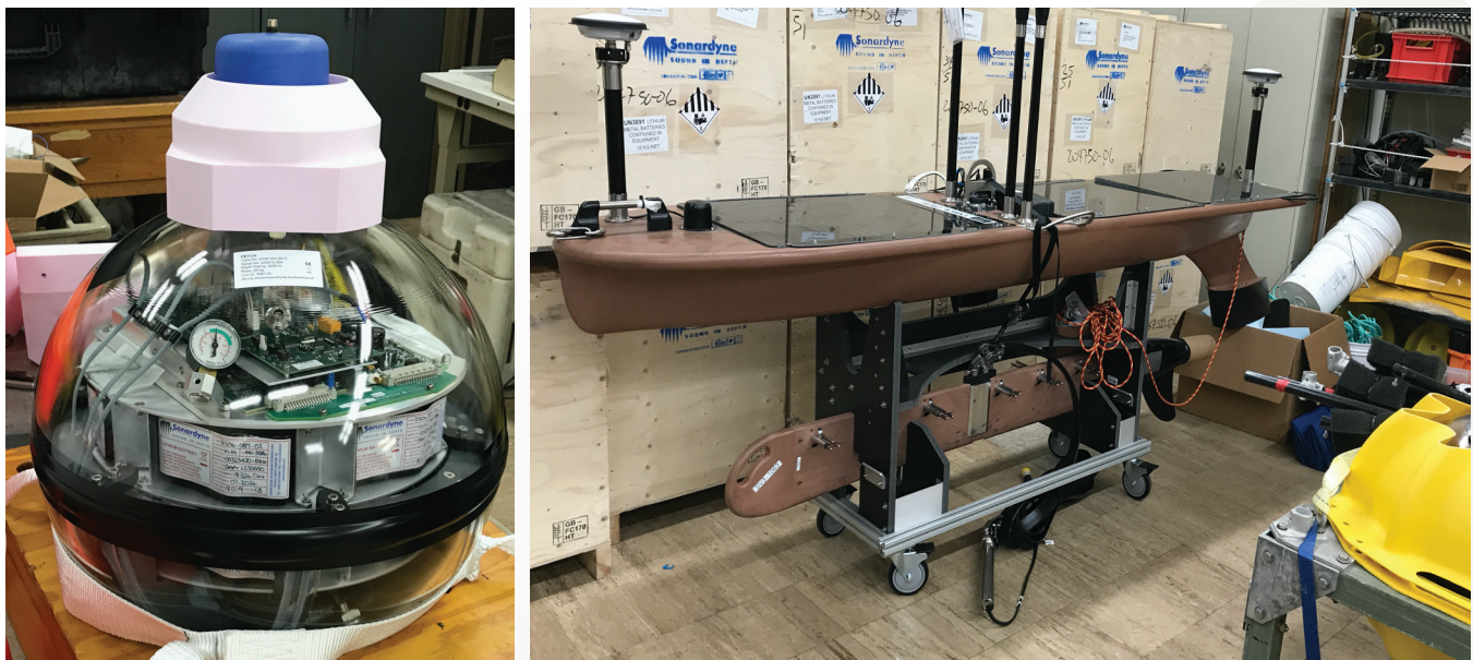
Figure 38. On the left is a Sonardyne seafloor transponder. It listens for coded acoustic pulses and replies with a unique pulse of its own. Measuring the round-trip time-of-flight of the pulses gives a measure of the distance between the transponder and the waveglider on the surface that initiated the connection. On the right is a Liquid Robotics SV3 waveglider, the latest generation vehicle available. It has been fitted with additional GPS antenna, an acoustic transducer, and inertial navigation sensors to equip it with GPS-A capability. Scripps has purchased 51 transponders, each with a 10-year battery pack, and three of the GPS-A wavegliders.
