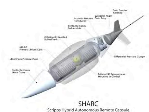
A second major goal of this MRI grant was to design an ocean bottom package capable of being self deployed – that is being towed out to the deployment site by a wave glider. Martin Rapa designed a prototype package, which we call the SHARC (Scripps Hybrid Autonomous Remote Capsule). Designed for a two-year bottom life, the SHARC is nearly 3 m in length and will weight about 650 Kg in air but is
