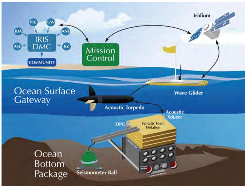
The overall concept is illustrated in the first figure. The wave-powered Wave Glider holds station over the ocean bottom package and acts as a surface gateway between acoustic transmissions through the ocean column and satellite transmissions to shore.
