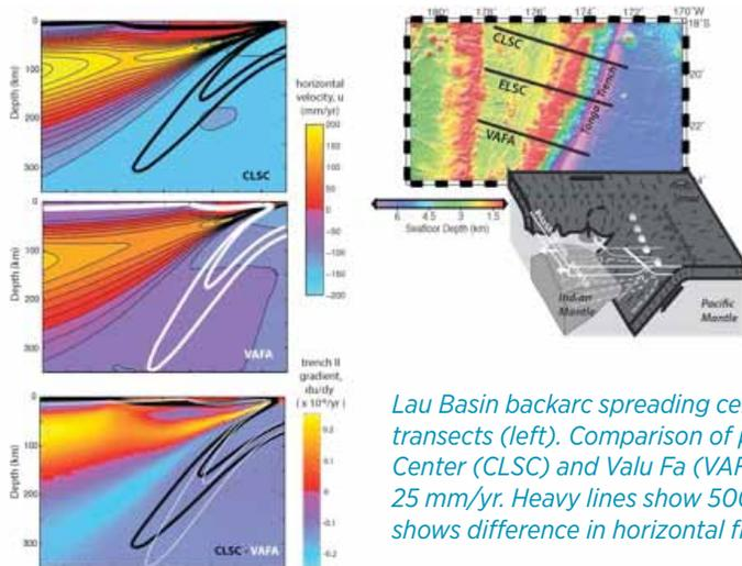
*Lau Basin backarc spreading centers (above, map and 3D sketch) and mantle wedge flow in three transects (left). Comparison of predicted horizontal component of 2D flow field at Central Lau Spreading Center (CLSC) and Valu Fa (VAFA). Top two panels have the same color scale for velocity, contour interval 25 mm/yr. Heavy lines show 500 °C and 700 °C isotherms for CLSC (black) and VAFA (white). Lower panel shows difference in horizontal flow between these models, scaled by distance between them.*
