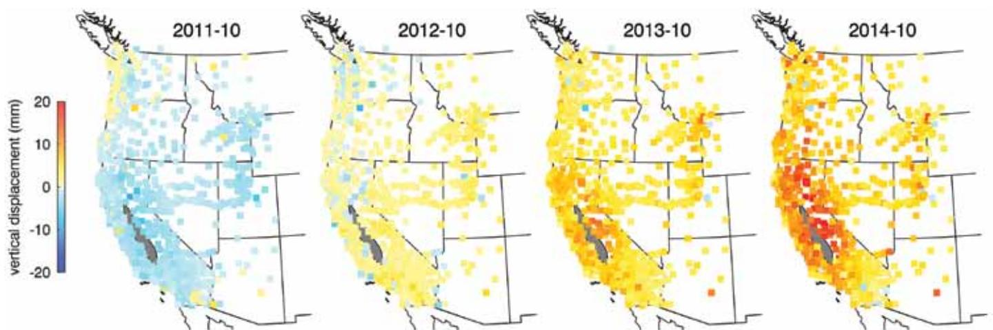
*Figure 1: Left: Spatial distribution of vertical displacements from Plate Boundary Observatory continuous GPS stations in the western USA in March of 2013 and 2014. Color indicates deviations of seasonally-adjusted elevations from decadal mean, with blues related to subsidence and yellow-reds related to uplift. Right: Mass load in mm of water equivalent derived from inversion of March 2014 vertical displacements, assuming elastic strains on a spherical Earth.*
