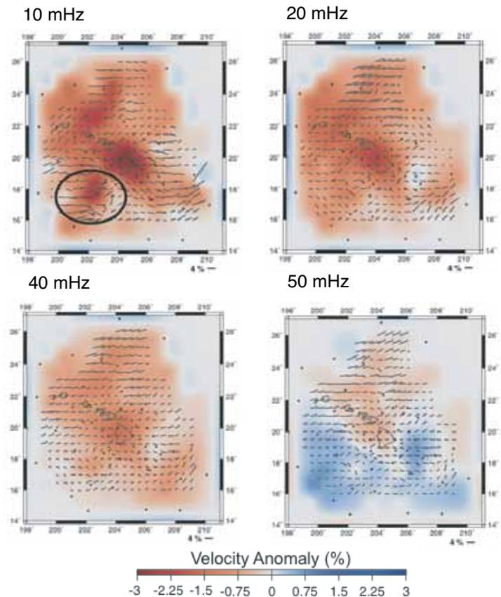
*Figure 1: Frequency-dependent Rayleigh-wave azimuthal anisotropy as observed during the PLUME deployments. Data were binned into  $1 \times 1^\circ$  cells. Higher frequencies are sensitive to upper-lithosphere structure, while lower frequencies reach into the asthenosphere. The signal for lower frequencies suggest that mantle flow in the asthenosphere is "disturbed" by plume-related upwelling.*
