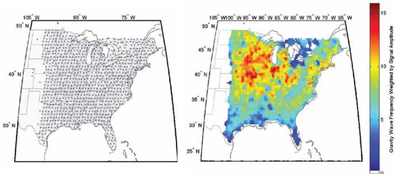
*Figure 1. left) sites occupied by stations in the TA from January 1, 2010 through Sept 30, 2014. These stations have been grouped into 3-element arrays (triads) for the study of long-period atmospheric gravity waves. The panel on the right shows the frequency of gravity waves in this time period with the count weighted by the amplitude of each detected wave. The most vigorous activity occurs to the west of the Great Lakes, as expected from satellite studies.*
