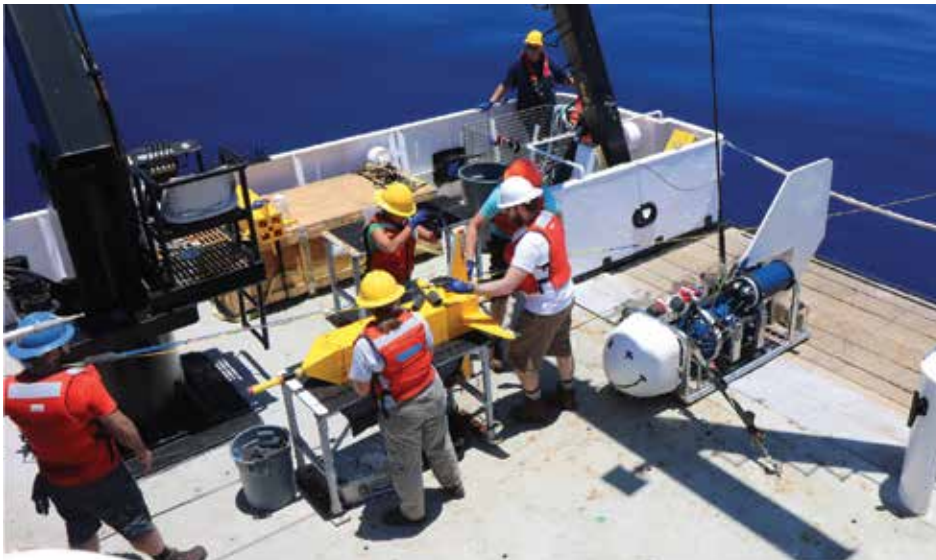
Figure 9. Preparing one of eight Vulcans (the yellow instrument) for deployment on a 1,600 m long array being towed behind our EM transmitter (SUESI with a smile) in the Gulf of Mexico. The entire system will be lowered to within 100 m of the seafloor to map gas hydrate.
