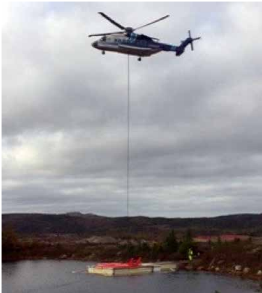
Figure 32. Test of an airborne earth-field NMR system for detecting near-surface contaminants. Image courtesy of ExxonMobil.
