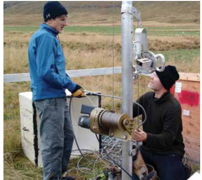
Figure 11. Dr. Carl Ebeling (left), IDA's chief engineer, and Bergur Bergsson (right) of the host Iceland Meteorological Office carefully lower a new seismometer package into the borehole at GSN station BORG (Borganes, Iceland).
