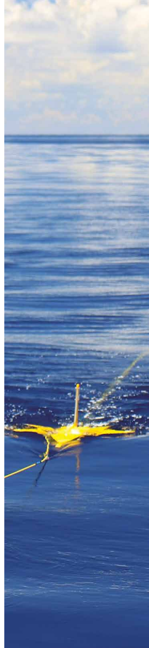
Figure 9. Preparing one of eight Vulcans (the yellow instrument) for deployment on a 1,600 m long array being towed behind our EM transmitter (SUESI with a smile) in the Gulf of Mexico. The entire system will be lowered to within 100 m of the seafloor to map gas hydrate.
