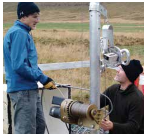
Figure 13. Dr. Carl Ebeling (left), IDA's chief engineer, and Bergur Bergsson (right) of the host Iceland Meteorological Office carefully lower a new seismometer package into the borehole at GSN station BORG (Borganes, Iceland). Photo courtesy C. Sites.
