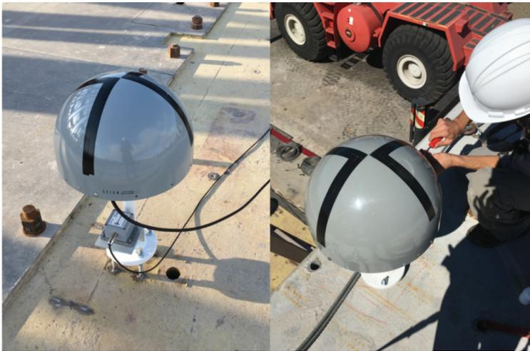
Figure 6. Installation of seismogeodetic instrumentation on a structure at the NHERI@UCSD Large High Performance Outdoor Shake Table. (Left) GPS antenna and SIO MEMS accelerometer on the shake table platen. (Right) On roof of the structure. The black tape on the antenna covers serves as targets for georeferencing UAV images of the structure. We use these earthquake simulations to test real-time data collection and earthquake detection algorithms.
