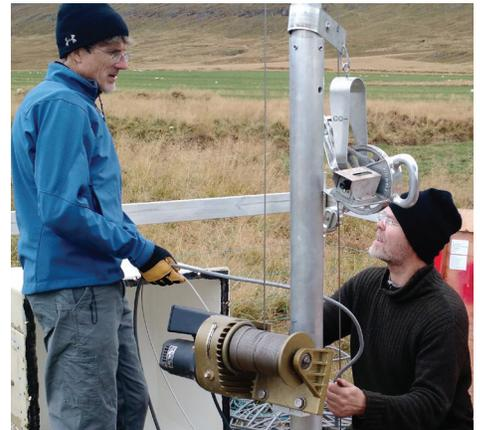
Figure 13. Dr. Carl Ebeling (left), IDA's chief engineer, and Bergur Bergsson (right) of the host Iceland Meteorological Office carefully lower a new seismometer package into the borehole at GSN station BORG (Borganes, Iceland). Photo courtesy C. Sites.
