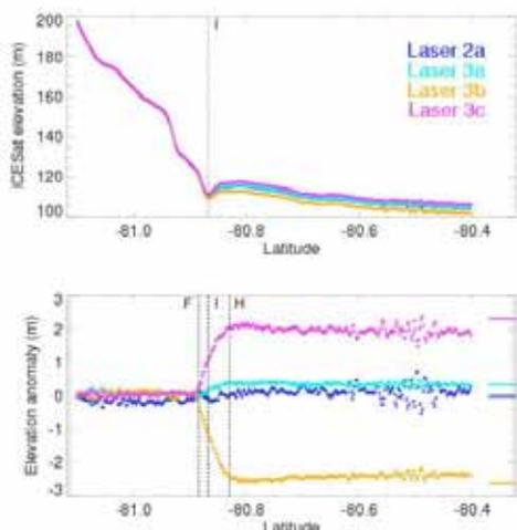
Figure 2. a) ICESat elevation profiles vs latitude for the four valid repeats of Track 218 and b) elevation anomaly values for each repeat. Horizontal lines at right are the equivalent anomalies based on tide predictions from a tide model. I is the break-in-slope; F is the limit of flexure and H is the seaward limit of the GZ.
