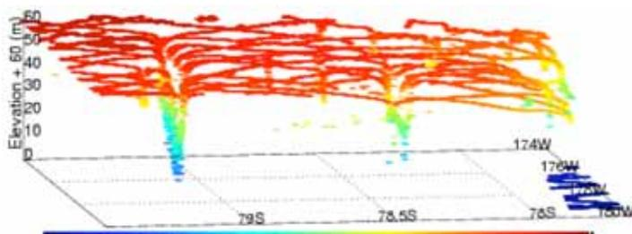
instruments have been integrated to monitor rift activity on Amery Ice Shelf, East Antarctica. These measurements have shown that rift propagation is episodic and occurs in discrete events separated by approximately 2 weeks.
