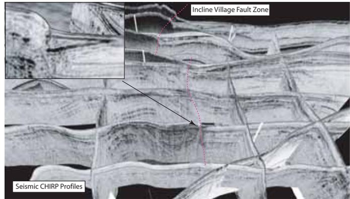
**Fig. 1** Seismic CHIRP profiles highlight fault structure (magenta), offshore Incline Village, view to the north. This crisscrossing network of profiles allowed proper identification of the Incline Village Fault scarp, which ran onshore and through the local elementary school, where the 7+ meter-deep trench was dug. Colluvial wedge from most recent event (MRE), 500 B.P., is seen in CHIRP profile (see inset).
