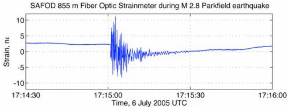
*Figure 2.* An optical fiber is stretched between the surface and a depth of 855 m in the SAFOD borehole near Parkfield, California. Small earthquakes on the nearby San Andreas fault cause deformations in the ground. This strain ( $\Delta z/z$ ) produces changes in the fiber optic cable's length, which is recorded by analyzing laser light transmitted through the fiber.
