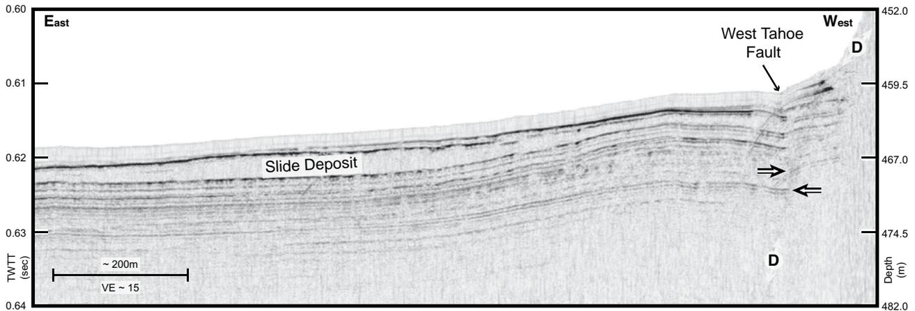
**Fig. 3** A seismic CHIRP profile showing the most recent rupture of the West Tahoe fault, along the west shore of Lake Tahoe. Arrows highlight at least 2-3 m of vertical displacement across sedimentary horizons, with lesser offsets near the lake floor indicating growth faulting. This seismic profile also images a distinct slide deposit that may have been triggered during this large event.
