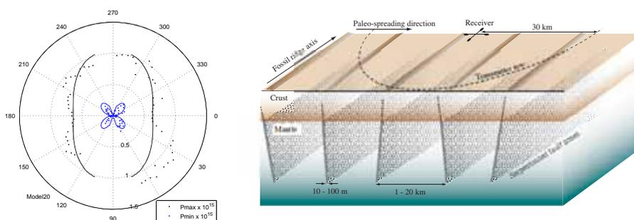
*Figure 1.* CSEM data from a circular transmitter tow around a central EM receiver, expressed as major (black) and minor (blue) axes of the polarization ellipse as a function of direction to the transmitter (left). The cloverleaf shape of the minor axis and the elongation of the major axis indicates anisotropy, which we model (solid lines) and interpret as serpentinized faults in the upper mantle (right).
