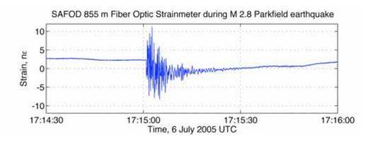
Figure 2. An optical fiber is stretched between the surface and a depth of 855 m in the SAFOD borehole near Parkfield, California. Small earthquakes on the nearby San Andreas fault cause deformations in the ground. This strain  $(\Delta z/z)$  produces changes in the fiber optic cable's length, which is recorded by analyzing laser light transmitted through the fiber.
