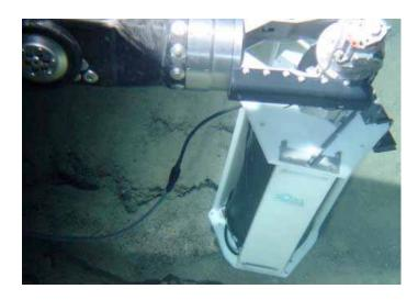
Figure 1. The ROVDOG instrument being deployed from the Nautile submersible. This image is from the expedition website, http://www.insu.cnrs.fr/web/article/art.php?art=1869.
